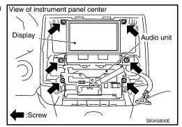
4. Remove screws and remove audio unit.
