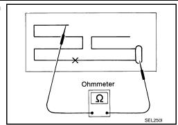
When measuring continuity, wrap tin foil around the top of probe. Then, press the foil against the wire with your finger.
