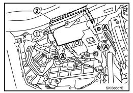
3. Remove TEL adapter unit screws, display control unit screws, and remove brackets.
