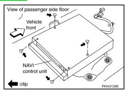
3. Remove screws (2) and nut (1) with power tool, and remove NAVI control unit.
