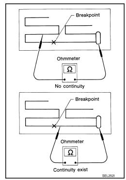
3. To locate a break, move probe along element. Tester needle will swing abruptly when probe passes the broken point.
