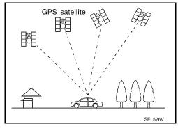
Position correction by GPS is not available while the vehicle is stopped.
