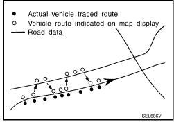
Map-matching does not function correctly when a road on which the vehicle is driving is new and not recorded in the DVD-ROM, or when road pattern stored in the map data and the actual road pattern are different due to repair.
