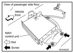
4. Remove screws (4) with power tool and remove brackets.
