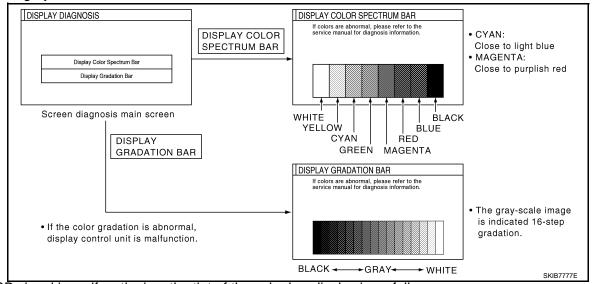
If RGB signal is malfunctioning, the tint of the color bar display is as follows.
