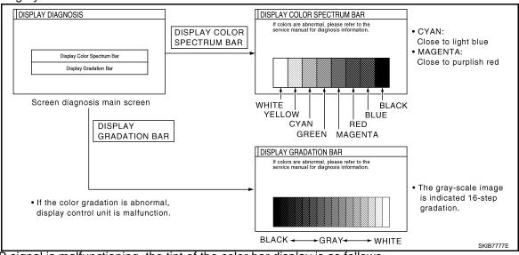
If RGB signal is malfunctioning, the tint of the color bar display is as follows.
