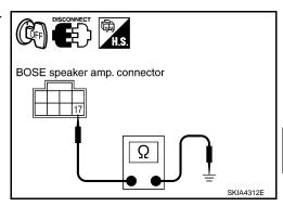
Check continuity between woofer harness connector B223 terminal 2 and ground.
