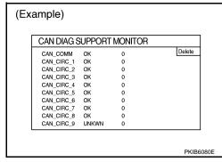
Record each item display description (OK/NG/UNKWN) displayed on the following CAN DIAG SUPPORT MONITOR Check Sheet.
