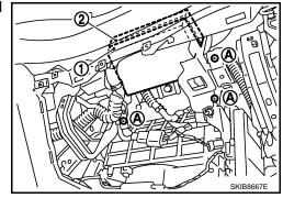
3. Remove screws (4) with power tool and remove brackets.
