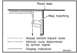
The vehicle position may not be corrected under the following circumstances and after driving for a certain time when GPS information is difficult to receive. In this case, the current-location mark on the display must be corrected manually.
