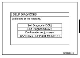
The transmitting/receiving of CAN communication can be monitored.
